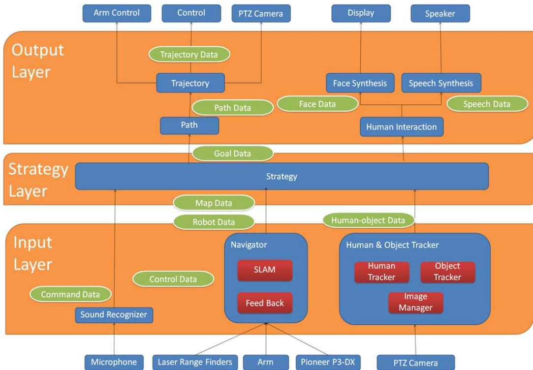
Figure 3 Software Architecture
