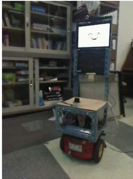
Figure 1: Robot with prototype structure which will be replaced by aluminum profile.
